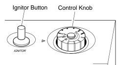
Figure 15 - Control Knob In The OFF Position
